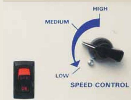
FIGURE 7 The flow rate on this machine is adjusted with the dial on the right-hand side.
