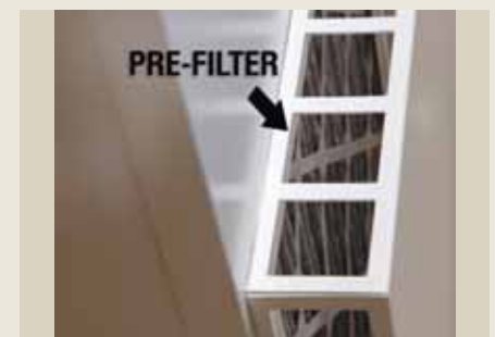
FIGURE 3 Pre-filter at inlet side of HEPA machine (is shown).
