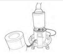
Use the Carbon Canister Lift Handle to remove the Carbon Cannister by gently pulling it directly up and out of the base Carbon and UV-C Housing Section. Discard the expired Carbon Canister.
