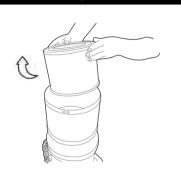
Remove HEPA canister filter from HEPA Canister Housing. Dispose of used HEPA canister filter per facility protocol for expired HEPA filtration materials.
