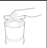
With all three (3) thumb screws removed lift top plate from HEPA Canister Housing to reveal HEPA canister filter.
