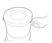
Note: HEPA Canister Housing Lid will be a snug fit as to apply downward pressure compressing the anti-leakage gaskets. Align the screw holes properly.
