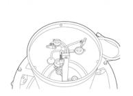
With all expired UV-C Light Bulbs removed from Light Array Assembly Posts, unit will will look like this. See illustration.
