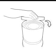
With replacement HEPA Filter Canister positioned properly level and closed Black Solid top of canister facing up, place HEPA Canister Housing Lid back onto HEPA Canister Housing,
