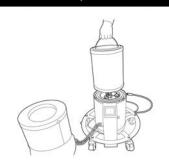
Using Canister Handle - slide New Replacement Carbon Canister into Carbon Canister Base Housing, Any position, as long as flat and level, will
