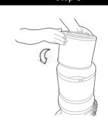
Position replacement HEPA canister filter in unit. Be sure to have the Black Solid closed top of HEPA canister filter facing upward with the filter canister open end facing down towards Motor Housing.
