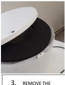
REMOVE THE BOTTOM COVER AND THE FOAM GASKET
