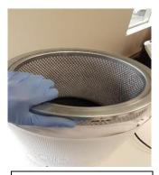
6. REMOVE THE CARBON FILTER BY FIRMLY PULLING IT OUT. THE PREFILTER IS HOLDING ON THE CARBON FILTER SO YOU HAVE TO OSCILATE THE MOVMENTS WITH BOTH HANDS IN ORDER TO RELEASE IT.
