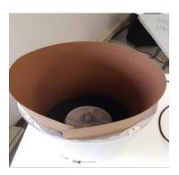
2. IN ORDER TO INSTALL THE CARBON FILTER, YOU NEED TO USE A THE PROVIDED SLIDER. PUT THE SLIDER INSIDE THE FILTER COMPARTMENT AND GENTLY SPREAD IT AGAINST THE PREFILTER
